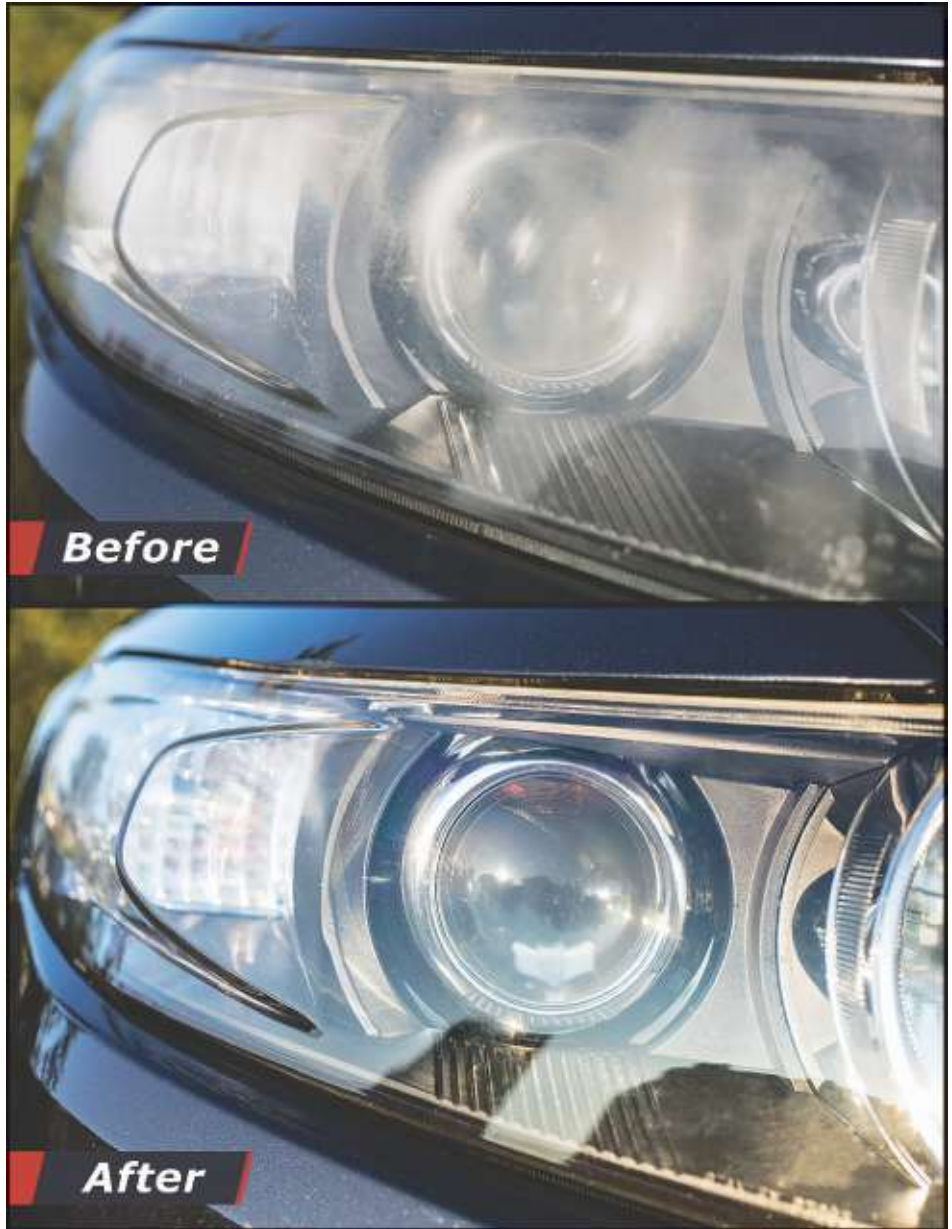
Polishing the optics of car headlamps. Effect Before and after the effect of polishing
